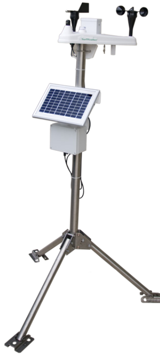
FIGURE 5-21. Auxiliary battery enclosure mounted to the 16776 tripod
