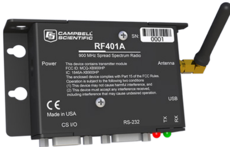
FIGURE 4-9. Radio connections. The serial cable connects to the RS-232 port and the AC adapter connects to the Power port.
