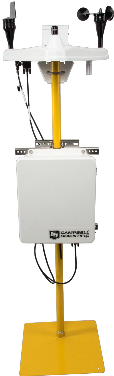
FIGURE 5-24. ATP100 enclosure and WS-PRO LT station mounted to pole
