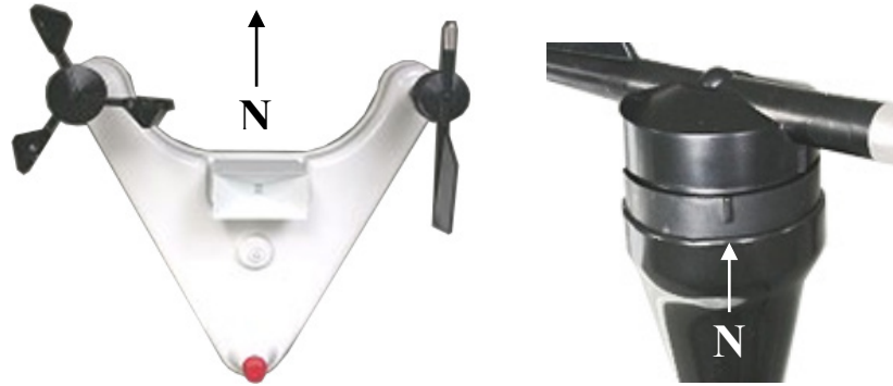
FIGURE 5-9. Accurate wind direction measurements require the reference line on the wind direction sensor (right) to be aligned with Magnetic North
