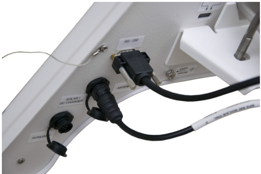
FIGURE 5-18. Short haul modem cables connected to WS-PRO LT station
