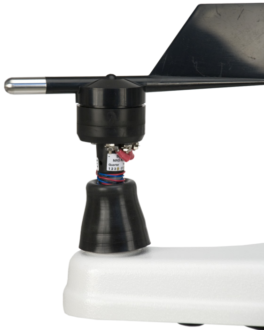
FIGURE 6-7. Wind direction sensor with boot down and exposing wires
