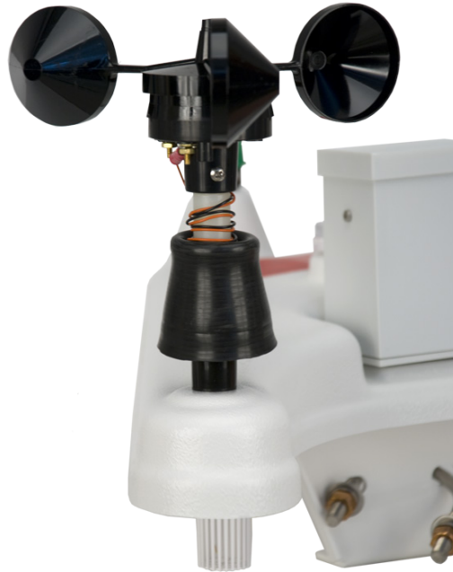
FIGURE 6-6. Wind speed sensor with boot down and exposing wires
